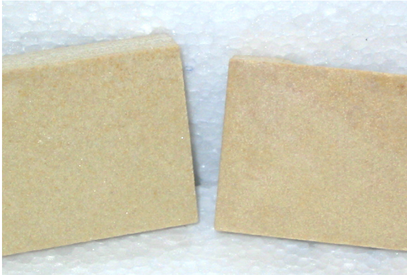
Honed sandstone sample comparison Pre and post sodium sulphate and chloride
