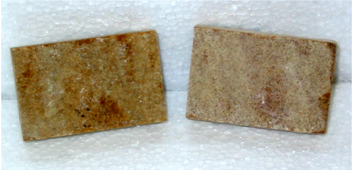
Exfoliated sandstone sample comparison Pre and post sodium sulphate testing
