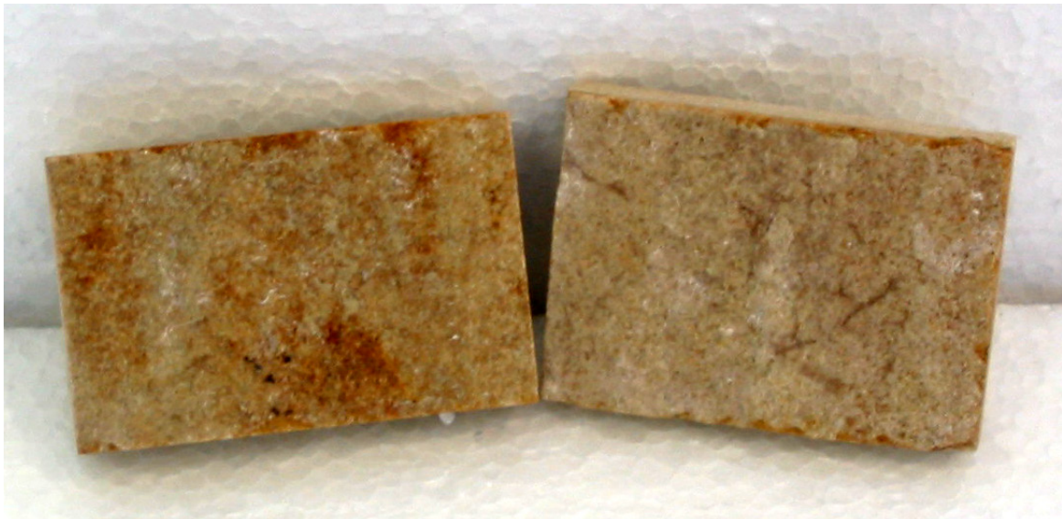
Exfoliated sandstone sample comparison Pre and post sodium chloride
