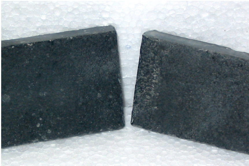
Basalt sample comparison. Basalt samples were only mildly affected by sodium chloride.
